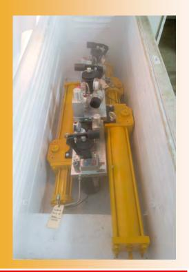
Each WCSCHP unit is frozen and tested for a MINIMUM of 24 HOURS to -30°C / -22°F
