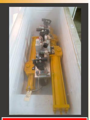
Each WCM Hydraulic Actuator Series Actuator is frozen and tested for a MINIMUM of 24 HOURS
