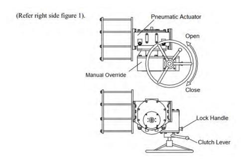
Release Hydraulic pressure. Operate worm hear as follows:
