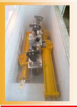
Each WCSCLP unit is frozen and tested for a MINIMUM of 24 HOURS to -30°C / -22°F
